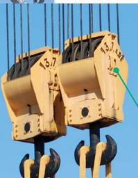
Full complement cylindrical roller bearings are located here in the vessel crane.
